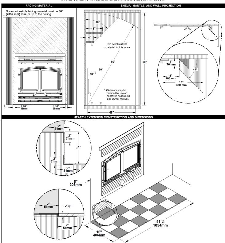
\*If fireplace is installed directly on the floor or on a raised base of less than 4", the hearth extension floor area must extend at least 16" (406 mm) in front of the fireplace with R-value equal to or greater than 1.00. Use 1/2" Micore or refer to manual for equivalent insulation.
