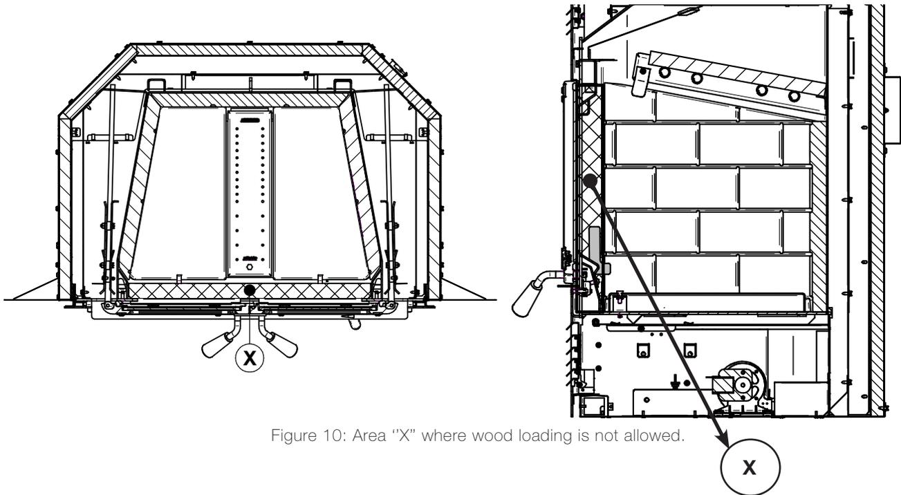
Figure 10: Area "X" where wood loading is not allowed.
