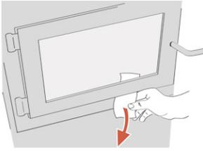
In order for the fireplace to burn at its best efficiency, the door must provide a perfect seal with the firebox. Therefore, the gasket should be inspected periodically to check for a good seal. The tightness of the door seal can be verified by closing and latching the door on a strip of paper. The test must be performed all around the door. If the paper slips out easily anywhere, either adjust the door or replace the gasket.
