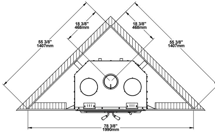
*Framing configuration should be used as a reference only.* If a finishing material is installed inside the enclosure, its thickness must be added to the following measurements. These values are minimum measurements and may need to be increased to allow the installation of the fresh air intake, the forced air kit or the type of finishing material used.
