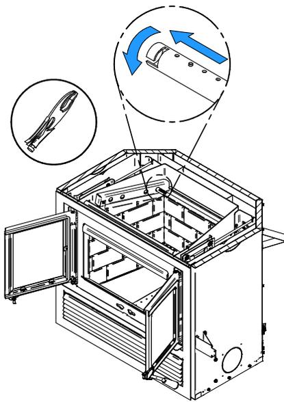
2. Align the notch in the left end of the tube with the key of the left air channel hole. Using a «Wise grip» hold the tube and lock it in place by turning the tube as shown. Make sure the notch reaches the end of the key way.
