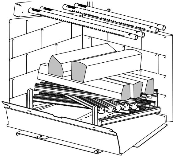
Figure 16: Start-up fuel configuration (over the kindling) -
