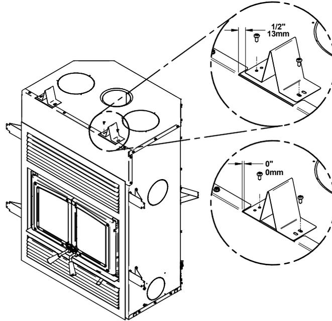
**Do not use combustible materials for the frame directly above the fireplace. This area should remain empty to a height of 80" (2032 mm) measured from the base of the fireplace.**
