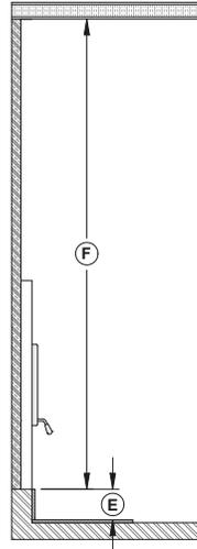
When the fireplace is installed on a raised base of less than 4" (101 mm) **(E)**, a non-combustible floor protection of at least 16" (406 mm) **(A)** with an R value of 1.00 must be installed in front of the fireplace.
