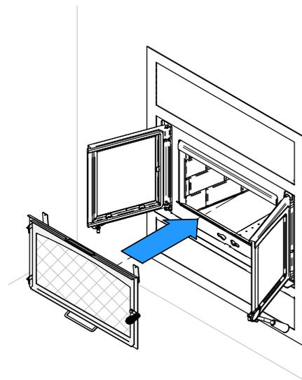
3. Lean the upper part of the firescreen against the top door opening making sure to insert the top firescreen bracket behind the primary air deflector.
