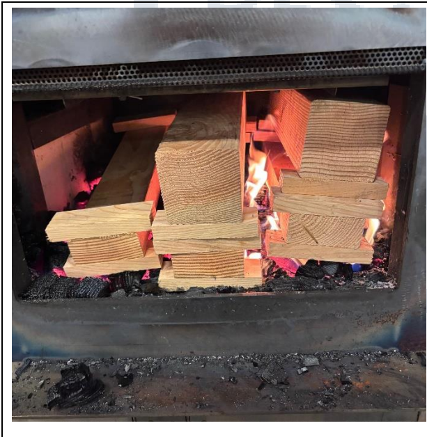
Test Fuel Loaded in Stove
