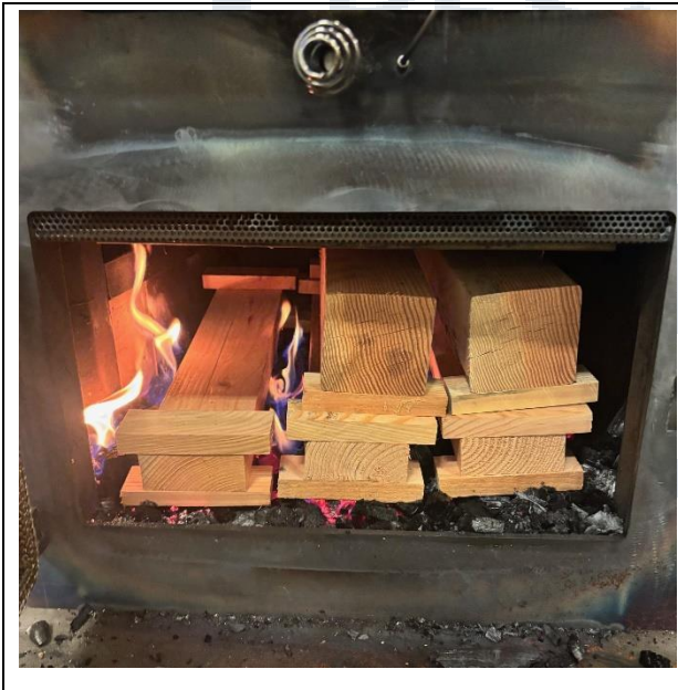
Test Fuel Loaded in Stove
