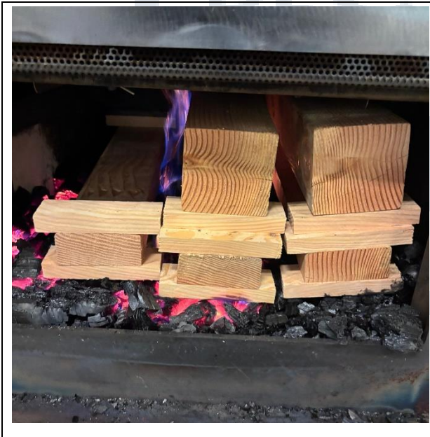
Test Fuel Loaded in Stove
