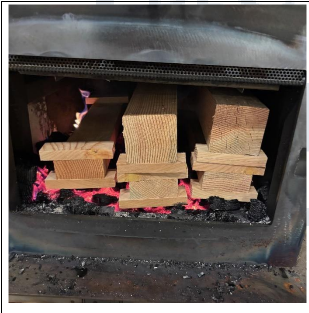
Test Fuel Loaded in Stove
