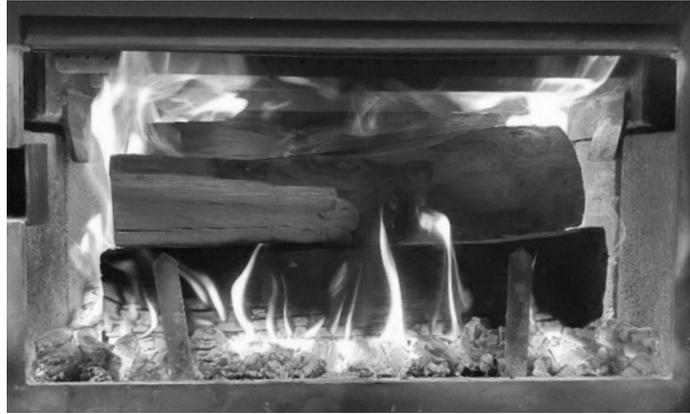
Close the primary air control by small increments (ex: 1/16 of an inch) until reaching the mid-point of air control position, between 4 and 15 minutes after the loading period. Before closing further, make sure the flame intensity is increasing or stable. Turn ON the blower at maximum speed
