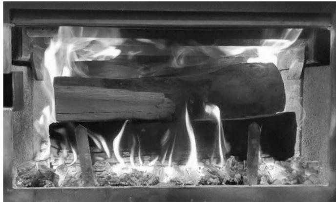
Close the primary air control by small increments (ex: 1/16 of an inch), from 1/2" to fully closed, between 4 and 15 minutes after the loading period. Before closing further, make sure the flame intensity is increasing or stable. Close the air control completely. Turn ON the blower at maximum speed.
