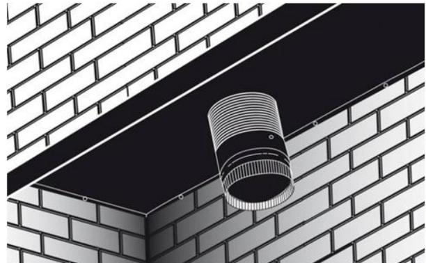
Figure 34: Block-off Plate
